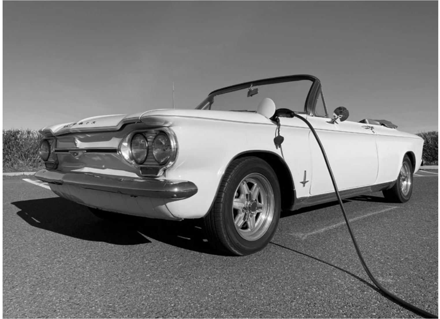
A 1964 Chevrolet Corvair that is now fully electric. Photo by Summer Schneider.
